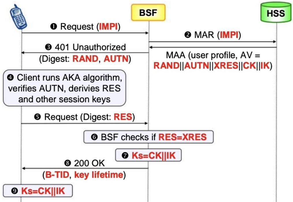
Figure 5-17 Bootstrapping procedure (GBA)
