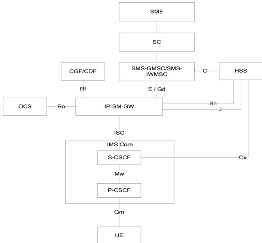
■ **Figure 5.1: Architecture for providing SMS over a generic IP-CAN**
