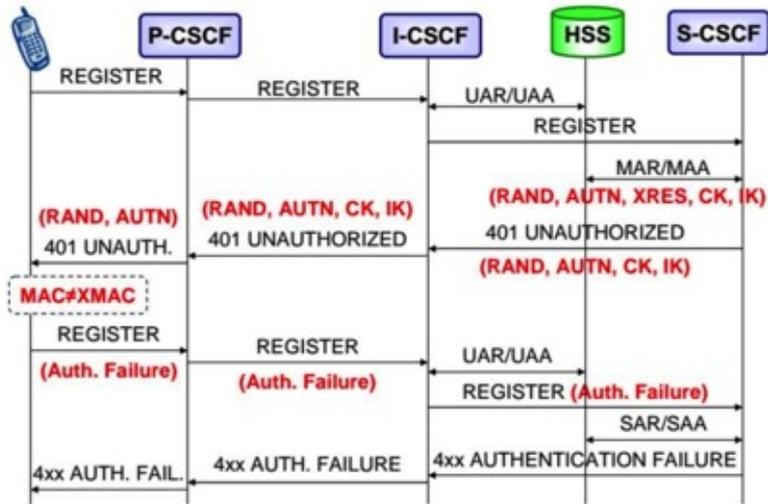
Figure 5-4 IMS AKA (network authentication failure)
