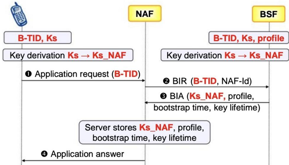
Figure 5-18 Bootstrapping usage procedure (GBA)
