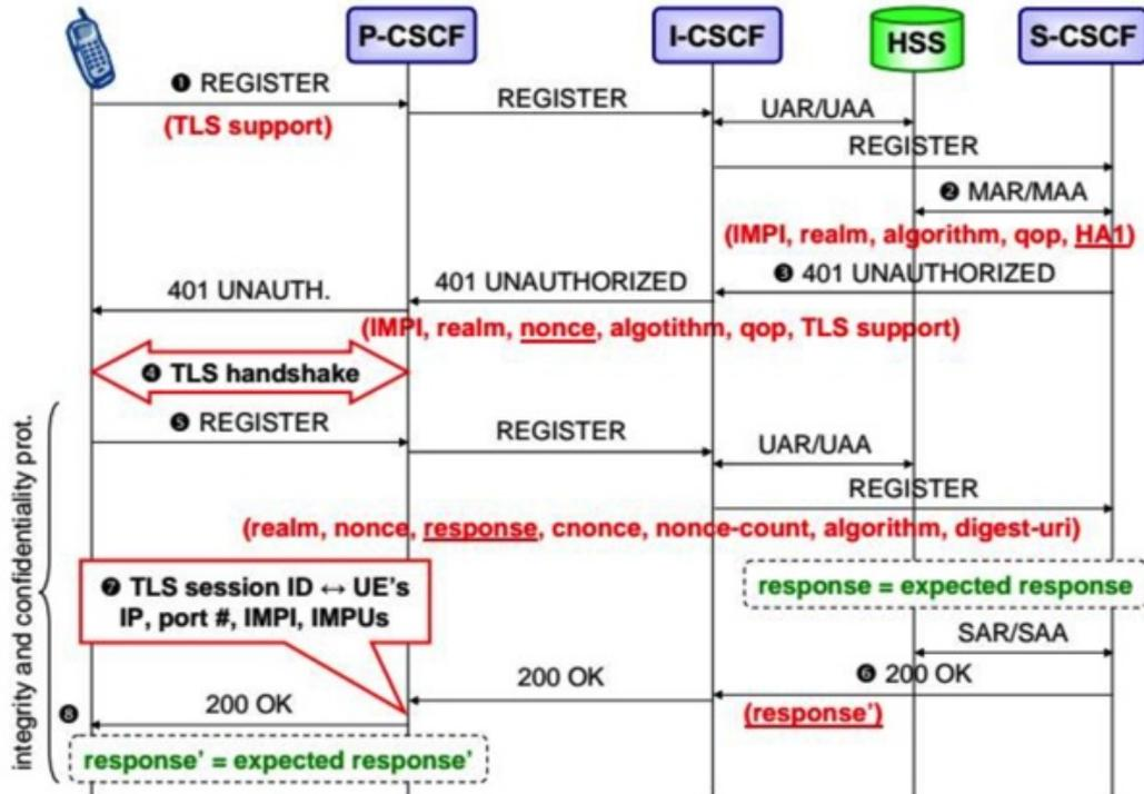
Figure 5-10 SIP Digest with TLS
