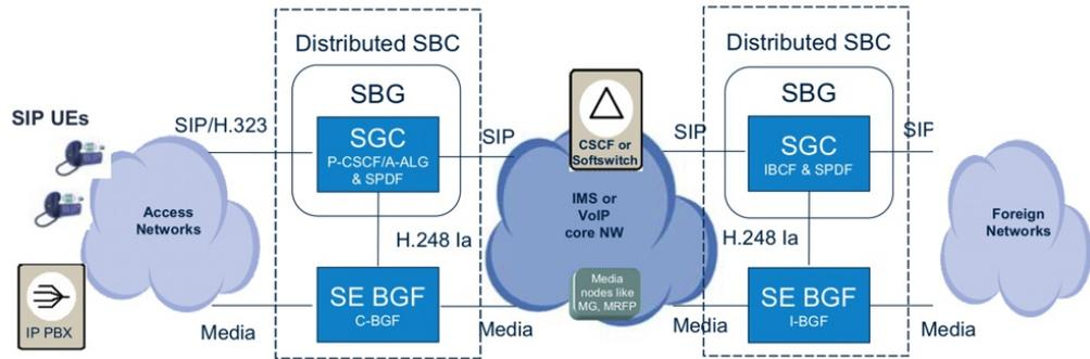
Figure 1 Logical Position of D-SBC and SmartEdge BGF in IMS or Other Multimedia Networks
