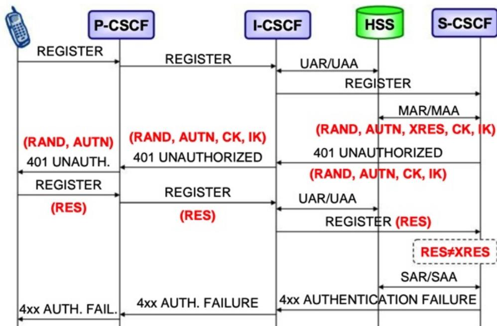
Figure 5-3 IMS AKA (user authentication failure)
