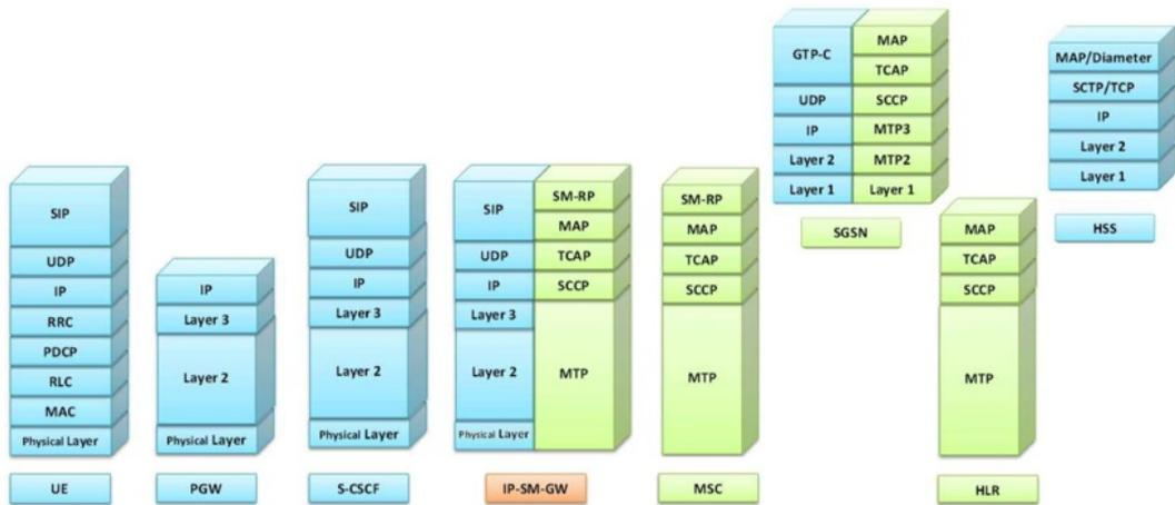
Figure 31. Service level interworking - Protocol Stack
