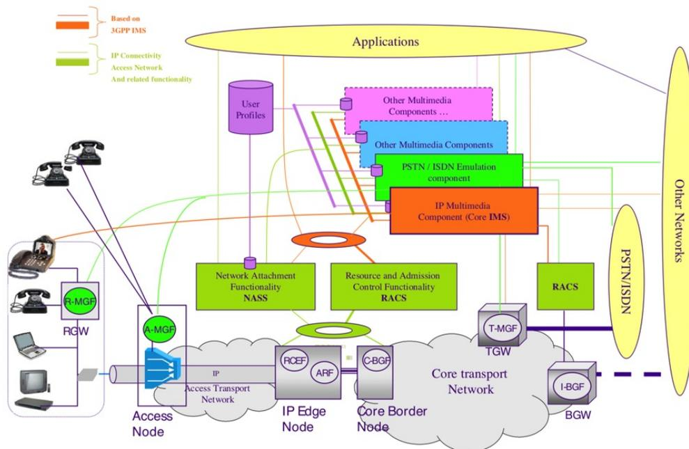
**Figure A.1: Example architecture with xDSL access**
