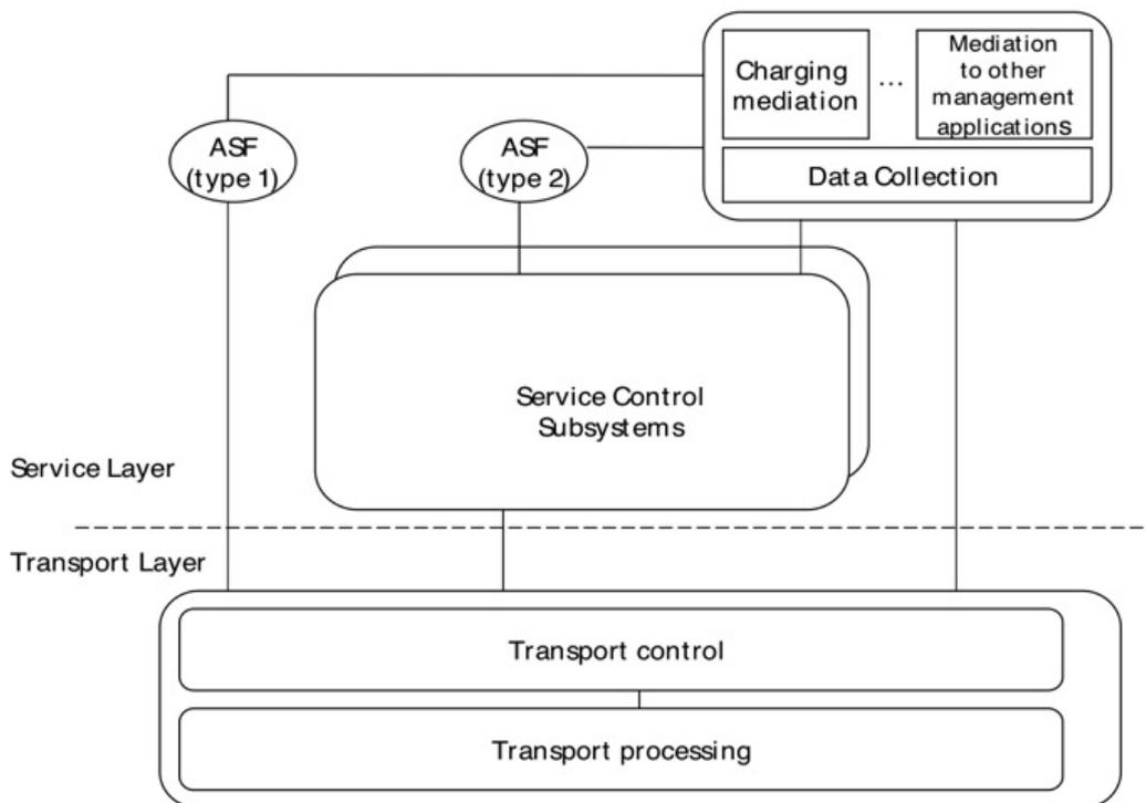
**Figure 4a: Charging and Data Collection Functions**
