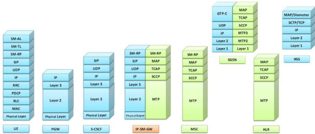
Figure 24. Transport level interworking - Protocol Stack
