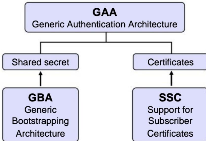
Figure 5-13 GAA mechanisms to issue authentication credentials
