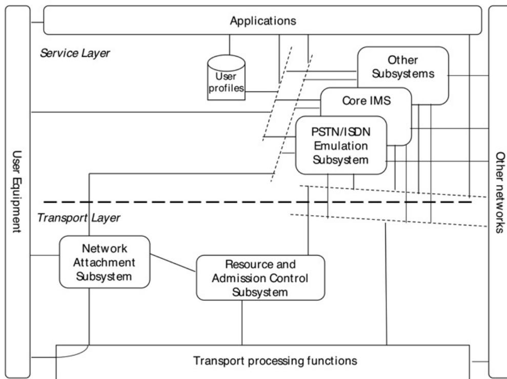
**Figure 1: TISPAN NGN overall architecture**
