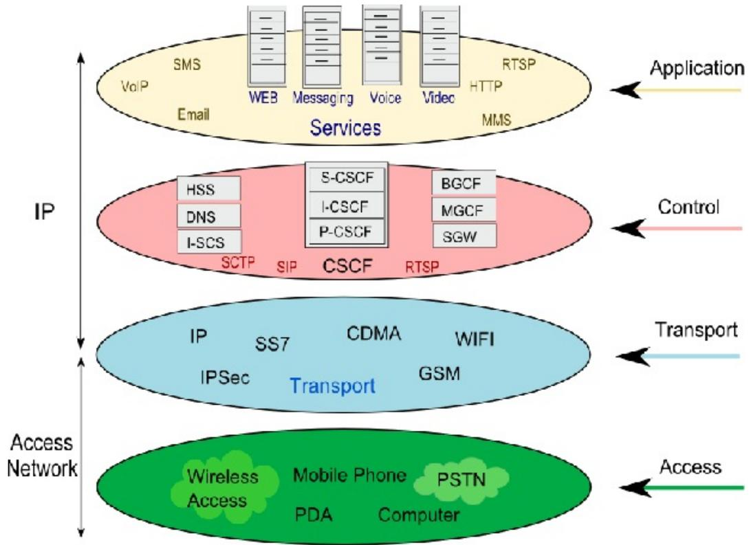
Fig. 2: IMS Network Architecture
