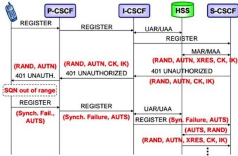
Figure 5-5 IMS AKA (synchronisation failure)
